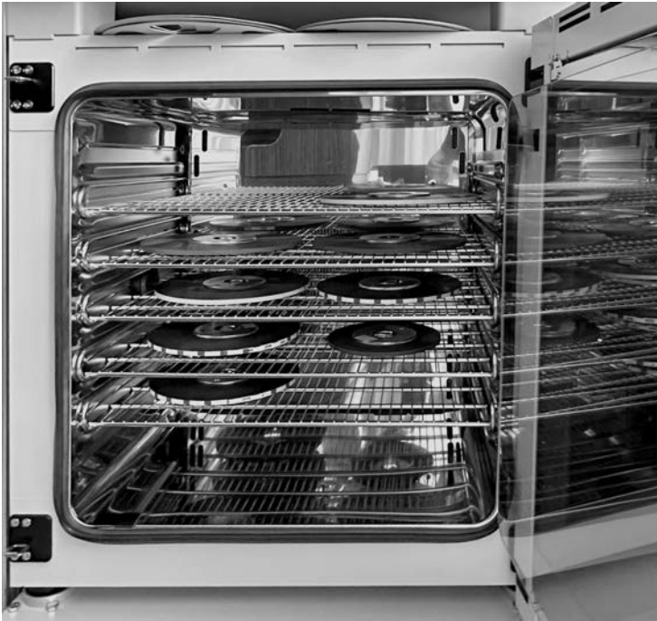
Figure 12. Some Pyral CJ87 tapes in one of the Binder BF115 lab incubators. Source: the author.
